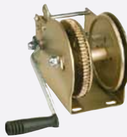
Ratchet winch (page 8) Reversible ratchet 1, 2 or 3 speeds. Removable handle.
