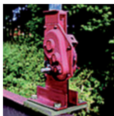
Single Sluice Gate drive
